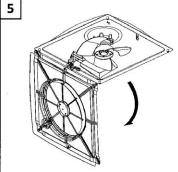
Gently allow the bottom housing to hang from the assembly connection on the oposite side.
