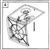
Turn the Blade Set Cap clockwise to remove the Blade Set
