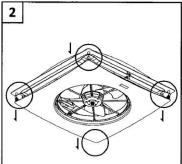
Unscrew (by hand) the four thumb screws located on the corners of the fan. The thumb screws do not come off, they remain secured to the fan by the plastic washers.
