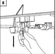
Disengage the connector by pressing on the thumb lock and gently pulling down.
