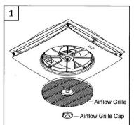
Turn the Airflow Grille Cap clockwise to remove the Airflow Grille
