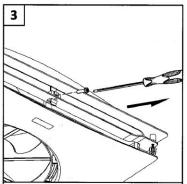
Use a Phillips screw driver to remove the screw from the safety bracket.
