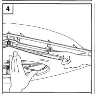
Disengage the safety bracket by supporting the bottom housing with one hand while using the other to press the safety bracket.
