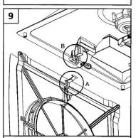
Gently push bottom housing upwards and disengage the pin bar "A" from the pin bar "B".
